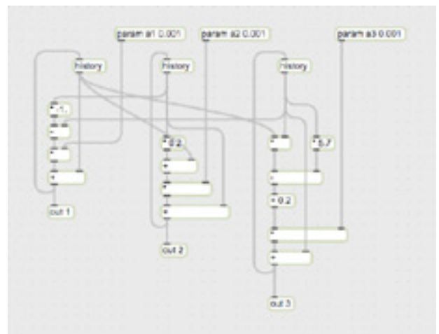
Figure 6. The rossler chaotic attractor built in gen~ by James, making use of the 1 sample delay
