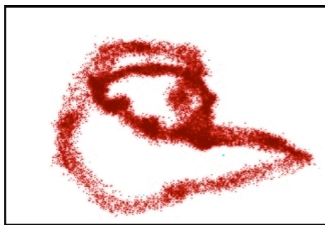
Figure 5. A quasi-periodic trajectory generated from an audio signal of a female singing at a fundamental frequency of 364Hz that was embedded in pseudo-phase space with a delay ( \tau ) of 485 samples; Generated by the author using Max/MSP/Jitter .
